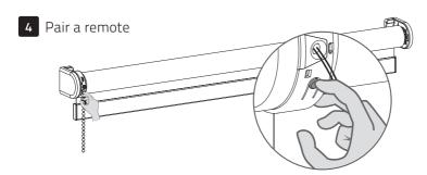
4.1 Shortly press the program button on the motor. The blind will start stepping, indicating that program mode has been activated.
